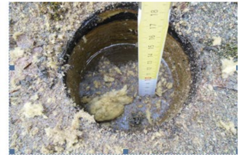
Foto 2: Boring 1 dakvlak- na 10min 5cm water in boring. Minerale wol is verzadigd
